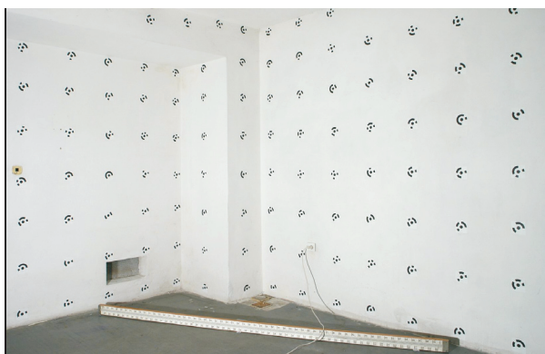
Fig. 3-1 The calibration and test field - CTF
