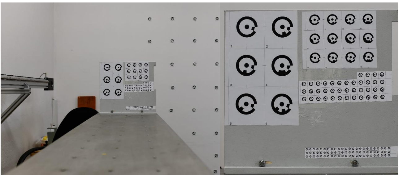
Figure 2: RAD target markers with a 50-, 25-, 10-, and 5 pixels inner disk diameter attached to a board fixed on the same panel as the camera (left-entire scene, right-closeup).
