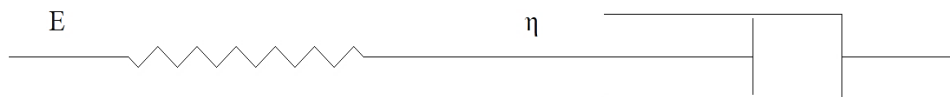
Figure 3: Graphical representation of Maxwell model \{M\}=(H) — (N) [7], where the Hookean spring is connected in series with the Newton's dashpot [3]
