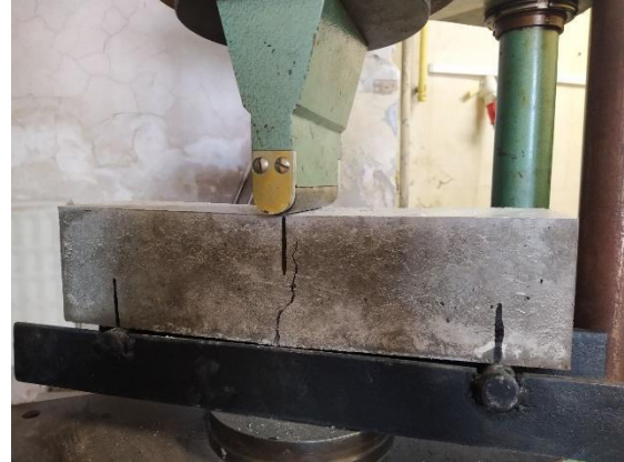
Figure 4: Testing of samples for flexural strength in bending
