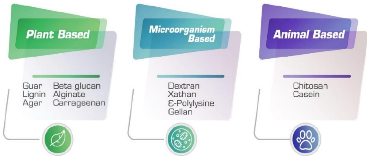
Figure 3: Common biopolymers used for soil improvement based on their production source. [18]
