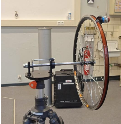
Fig. 4.4 – Prototype of the kinematic field testing equipment on the tripod
