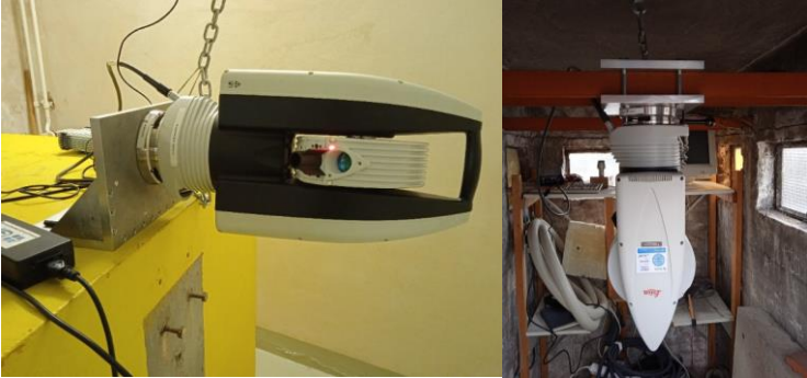
Fig. 4.3 –LT horizontal mounting (left), upside-down LT mounting (right)
