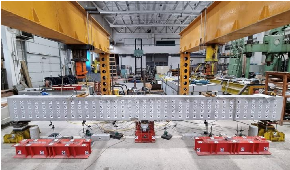
Figure 4.13 Test setup of continuous beams
